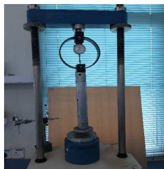
Figure 5: UCS testing machine.
