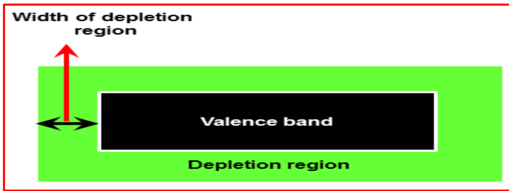
Figure 1: 2-D view of the depletion region in presence of atmospheric oxygen.
