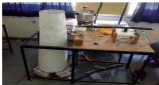
Figure 13: Cooling Tower with Condenser
