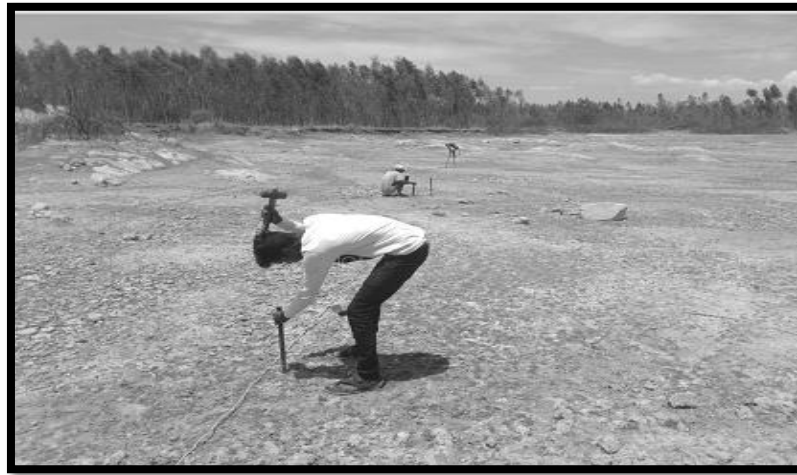
Figure 3: Field Work Data Collection and Electrode Layout
