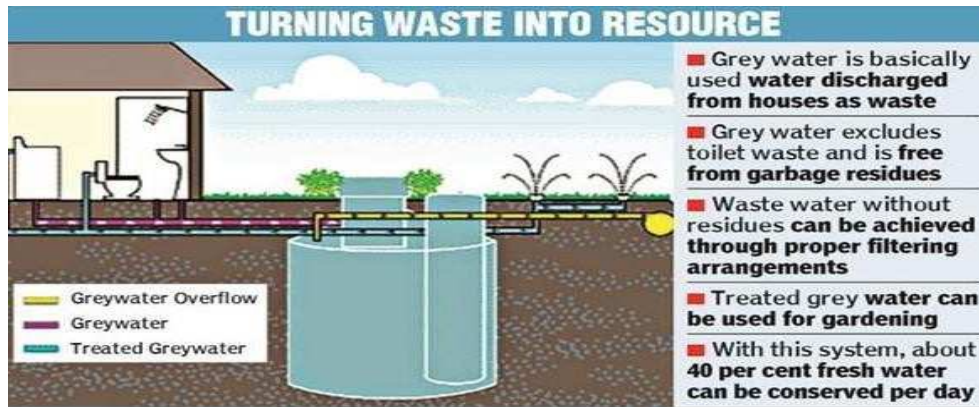
Figure 2: Grey water purification [32]
