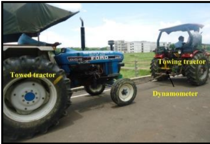
Figure 1: Slip Measurement with Towing and Towed Tractor
