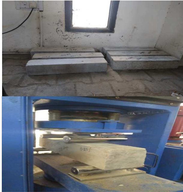
Figure 4: Testing of beam specimens.
