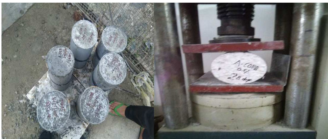
Figure 5 : Testing of cylinder specimens.
