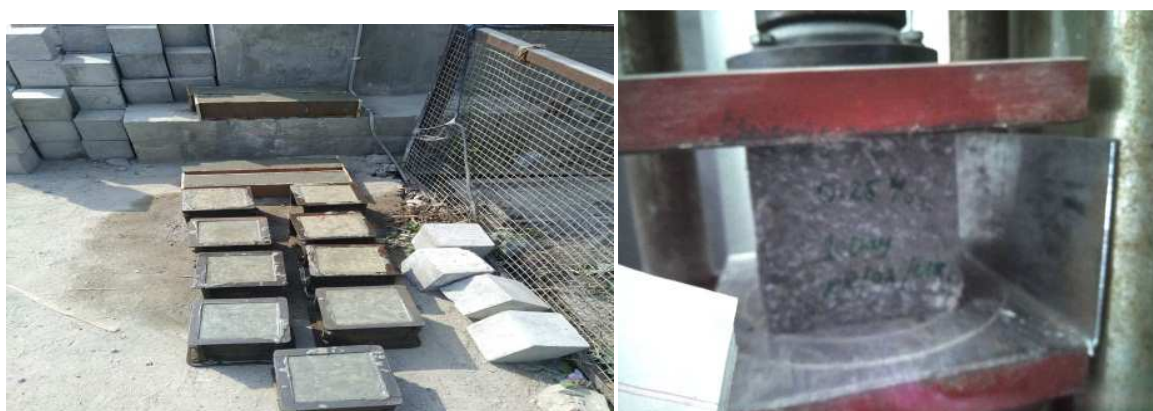
Figure 3: Testing of cube specimens.
