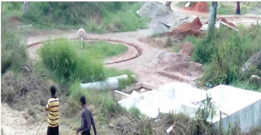
Figure 7: Showing Traditional lime mortar mill with adjacent slaking tank
