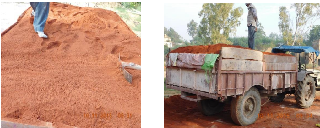
Figure 3: Showing Surkhi as raw material
