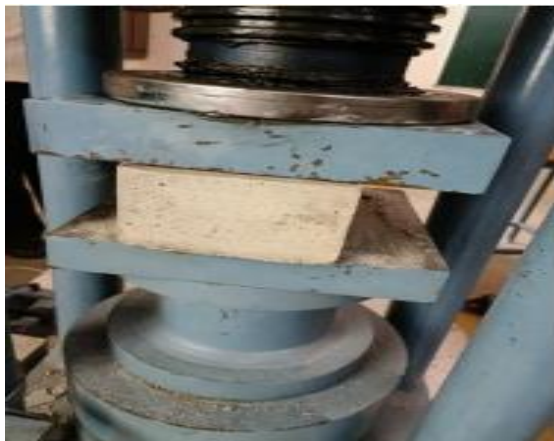
Figure 1: Compressive Strength Test on Concrete Cube
