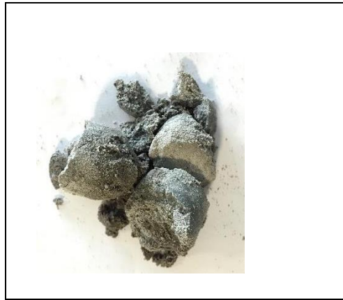
Figure 5: Ratio of diluted resin to silica fume, 1:1.5.
