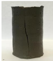
Diluted resin (resin + 30% of acetone) to fly ash, 1:1.0.
