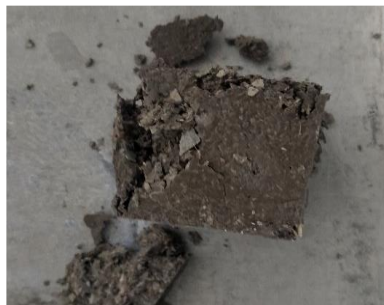
Figure 9: Crushing pattern of 50mm cube during compressive strength test for 2-hour age sample. Figure 10: Crushing pattern of 50mm cube during compressive strength test for 14-day age sample.
