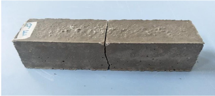
Figure 12: Crushing pattern of 50x50x200mm beam during flexural strength test using 14-day age sample.
