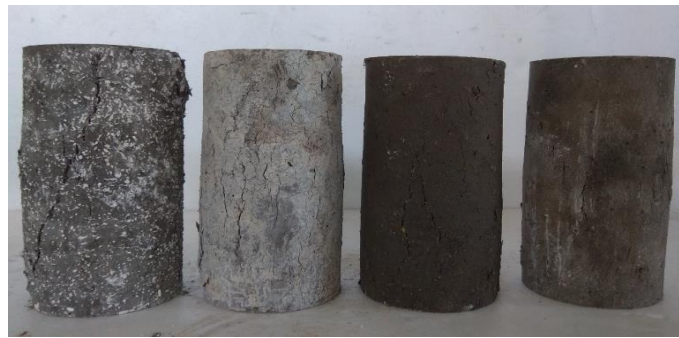
Figure 7: Surface of polymer concrete (100mm dia X 200mm height cylinder) after removing from aggressive solutions (from left to right: H 2 SO 4 , NaOH, NaCl, and Water).
