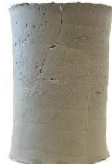
Diluted resin (resin + 30% of lacquer thinner) to fly ash, 1:1.0.
