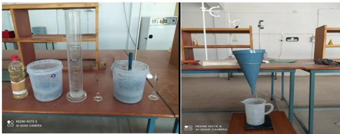
Figure 1: Cement, PCE, SMF, Marshcone Setup
